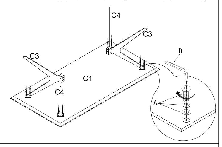
STEP 2:Use the Hex Key(C) to tighten the Legs(C3,C4) to the Leg Rail Panel(C2) with T Nut(B).
