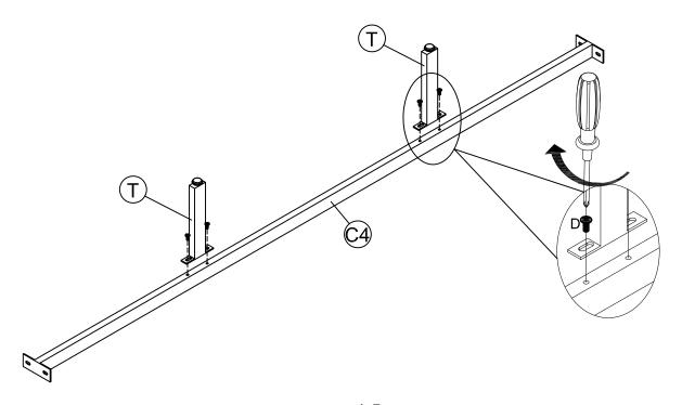
STEP 3: Use Hex Key to tighten Centre Rail(C4)to the Headboard (C1)and Footboard (C3)with Bolt(D)
