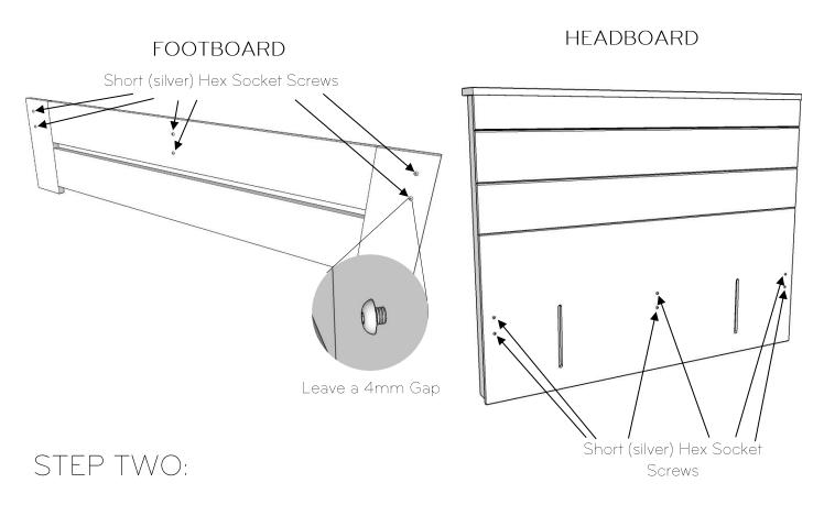
Take one of the Side Rails and slot the keyhole shape holes in the metal bracket over the two Screw Heads in the Footboard. The Side Rail should 'click' down into place. Then use the Allan Key provided to tighten the screws firmly.
