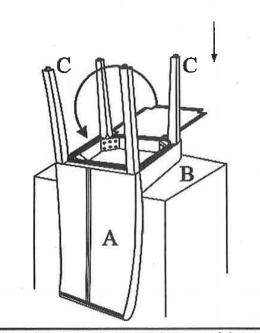
Place the Vinyl Flap to the bottom of the Seat (B), using the adhesive strip as shown.
