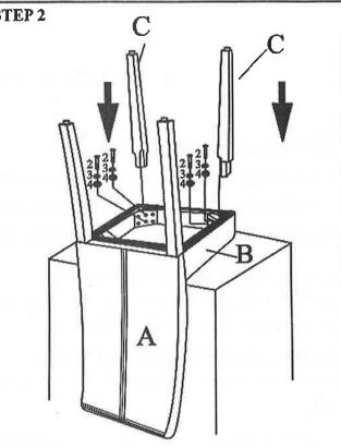
Attach the Seat (B) to the Chair Back (A) using four Long Bolts (1), two Short Bolts (2), six Spring Washers (3) and six Flat Washers (4), and with the provided Allen Key (5).
